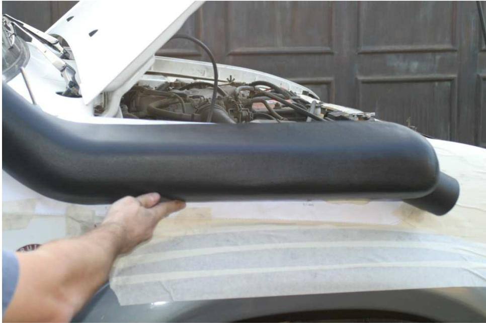
Before you drill make sure there is nothing on the other side that can be damaged, like wiring etc. Drill the marked holes. Do not press to hard, let the drill do the work, go slowly as the fender metal is very thin.
