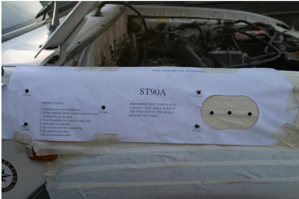
Using a jig saw with a fine metal cutting blade, cut out the large hole in the fender. Safety: Work slowly, wear safety goggles, and do no rush. Do not remove the blade from the fender until the jigsaw has stopped moving.
