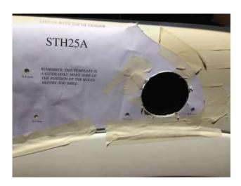
I tried to insert the snorkel and found the hole to be about 7mm to small and started filing the edges until it fitted. I made sure that the S pipe fitted neatly and aligned to both the inner and outer holes.
