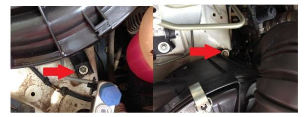
Remove the air filter housing. You will now notice the clips I mentioned before, these can be removed with long nose pliers by squeezing the little fins on the corners and pushing it down. There are 4 of them and take care when they fall out the bottom as to where it goes else you'll have to replace them. Also note on the inside of the fender where they were as this will help in re-assembly
